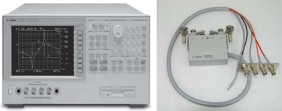
Figure 4: Impedance analyzer and connectors used to extract capacitance curves from the Pseudo-MOSFET samples.
