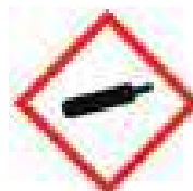
Gas under pressure
